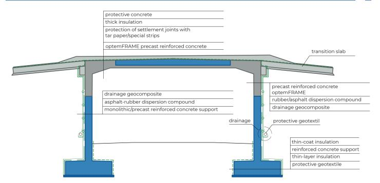
The monolithic lock not only has a connecting function, but also reduces the weight of the precast element. This has a significant impact on the efficient assembly of the elements on site and the transport of the precast elements.
