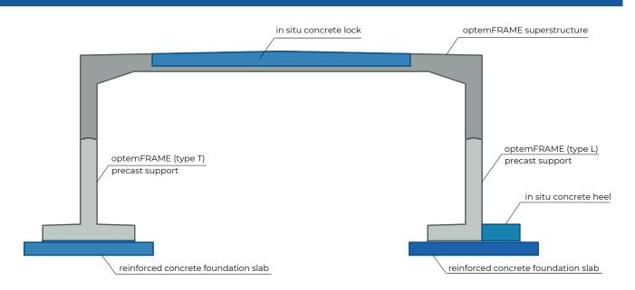
In comparison with monolithic supports, the use of precast frame elements and supports significantly reduces construction time. The connection between the precast superstructure elements and the supports was designed to ensure an easy on site assembly. The idea of the tongue and groove system allows for maintaining centric position and precise placement of the frame elements on the supports.
